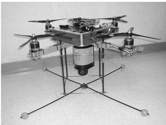
Fig. 15 Line-scan LADAR mounted within the carbon-fiber frame.
