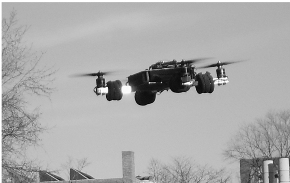
Fig. 14 Initial flight configuration without the carbon-fiber frame.
